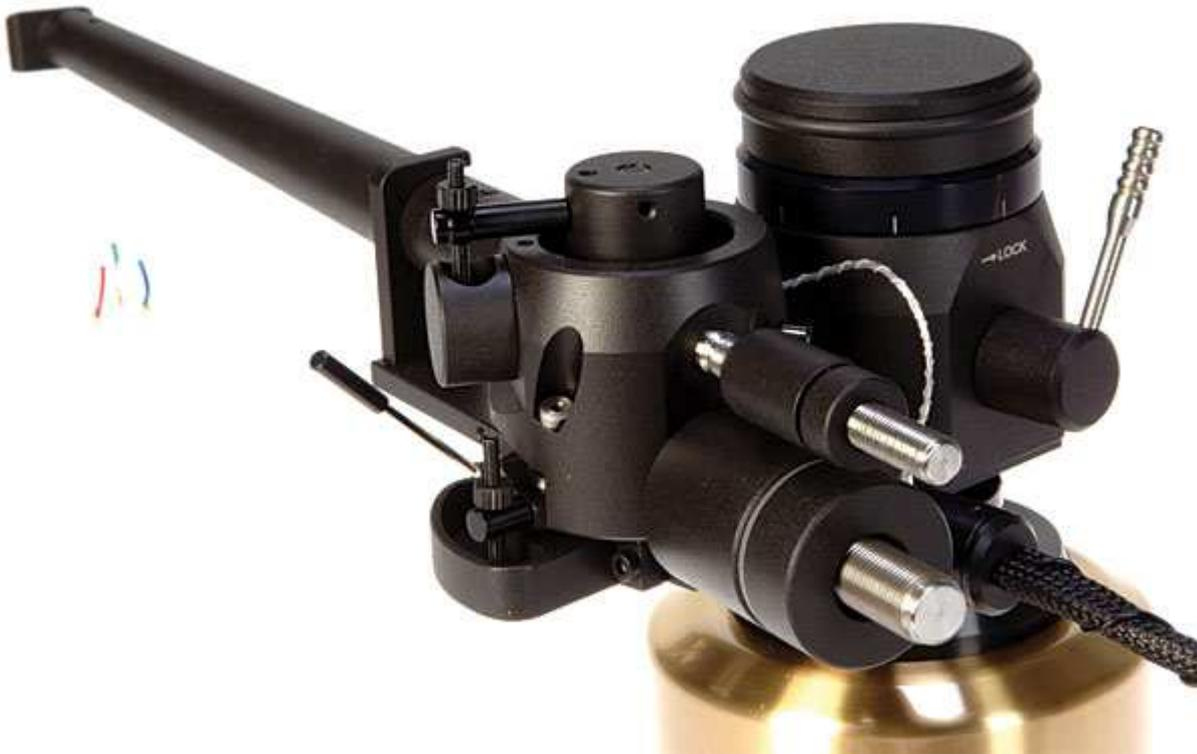
Also borrowed from the Airline is the 4Point's rigid, angled-construction headshell—but this one is removable, thanks to a short, beefy, hexagonal protrusion that fits securely into a matching opening on the arm and locks tightly with a grub screw atop the arm. A tiny threaded hole lets you screw in the finger lift, if you want it.
